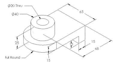
As an aid to constructing this part, visualize how it could be broken down into individual features:
